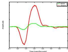
Figure 1 : Typical waveforms reflected by normal and malignant tissue types.
